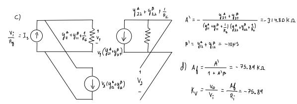
$$A' = -\frac{y_{21}^{A} + y_{21}^{B}}{(y_{11}^{A} + y_{11}^{B} + \frac{1}{R_{6}})(y_{22}^{A} + y_{22}^{B} + \frac{1}{R_{6}})} = -3 + 4.80 \text{ K}.$$
