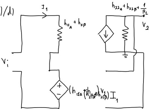
$$A' = \frac{V_2}{V_1 A} = -\frac{h_{21A} + h_{21\beta}}{(h_{11A} + h_{11\beta})(h_{22A} + h_{22\beta} + \frac{1}{R_L})} = 3865$$
