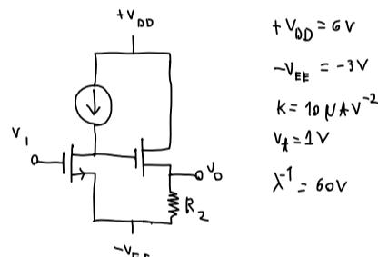
$$\begin{aligned}+V_{DD} &= 6 \text{ V} \\-V_{EE} &= -3 \text{ V} \\k &= 10 \text{ mA/V}^{-2} \\V_t &= 1 \text{ V} \\X^1 &= 60 \text{ V} \\I_D &= k(-V_{GS} - V_t)^2 = 40 \mu\text{A} \\I_A &= I_D = 40 \mu\text{A}\end{aligned}$$
