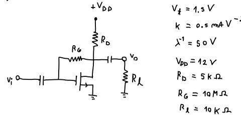
$$\begin{aligned}V_t &= 1.5 \text{ V} \\k &= 0.5 \text{ mA/V}^{-2} \\X^1 &= 50 \text{ V} \\V_{DD} &= 12 \text{ V} \\R_D &= 5 \text{ k}\Omega \\R_G &= 10 \text{ M}\Omega \\R_L &= 10 \text{ k}\Omega\end{aligned}$$
