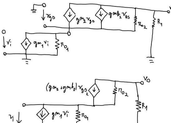
$$b) I_1 = I_{D1} = I_{D2} = I_{S1} = I_{S2}$$
