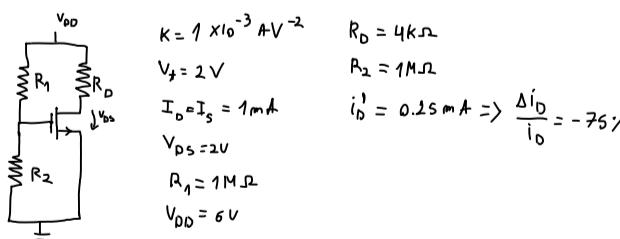
$$v_{DD} = R_D i_D + v_{DS} \Leftrightarrow \frac{v_{DD} - v_{DS}}{R_D} = R_D = 4k\Omega$$
