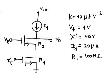
$$\begin{aligned}k &= 10 \text{ mA/V}^{-2} \\V_t &= 1 \text{ V} \\X^1 &= 50 \text{ V} \\I_1 &= 20 \mu\text{A} \\R_1 &= 100 \text{ M}\Omega \\G_m &= \frac{i_o}{v_i} \Big|_{v_o=0} = g_m = 2\sqrt{kI_1} = 28.28 \mu\text{s}\end{aligned}$$
