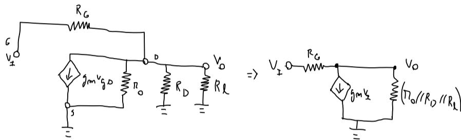
$$\begin{aligned}R_i &= R_G i_g + (R_D // R_L) i_R \\i_g &= g_m v_i + i_R \\v_i &= i_g R_i + v_o \Rightarrow v_o = v_i \left(1 - \frac{R_i}{R_o}\right) \Rightarrow A_v = \frac{v_o}{v_i} = -5.6 \\i_g &= \frac{v_i}{R_i}\end{aligned}$$
