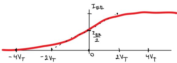
$i_{c1} = \frac{I_{FE}}{1 + \frac{i_{c2}}{i_{c1}}}$   $\Leftrightarrow i_{c1} = \frac{I_{FE}}{1 + e^{-\frac{v_I}{V_T}}}$
