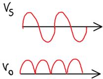
$$V_{o,av} = \frac{2}{T} \int_0^{T/2} A \sin(2\pi f t) dt = \frac{2A}{\pi} = \frac{10}{\pi} = 3.1831 \text{ V}$$
