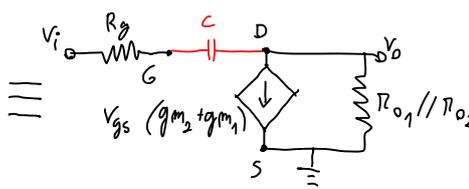
$A_v = \frac{V_o}{V_i} = - (R_{o1} // R_{o2}) (g_{m2} + g_{m1}) = -133.33$
