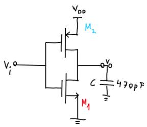
$$i_c = C \frac{dV_o}{dt} \Rightarrow \bar{i} \approx C \frac{\Delta V_o}{\Delta t} \Rightarrow \Delta t = \frac{C}{\bar{i}} \Delta V_o$$
