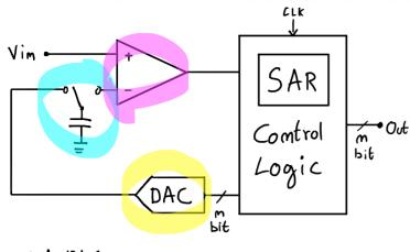
12 to 18 bits 500 kHz to 10 MHz A SAR ADC (or voltemeter) works by successively comparing the input voltage to a given voltage, generate in a binary search style.
