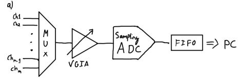
Multiplexer (Mux): Allows to select which channel will be adquired, and if single or differential mode.
