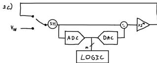
Equal to the other one but instead of having several stages, it uses only one stage and used feedback to always use that same stage.
