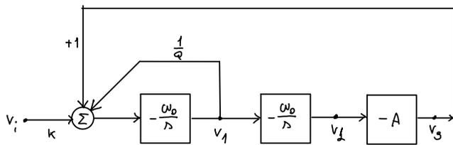
$$T_1: V_1 = -\frac{\omega_0}{\delta} \left( \frac{V_1}{Q} + V_3 + kV_i \right) \quad \begin{cases} V_3 = -AV_2 \\ V_2 = -\frac{\omega_0}{\delta} V_1 \end{cases} \Rightarrow V_3 = A \frac{\omega_0}{\delta} V_1$$
