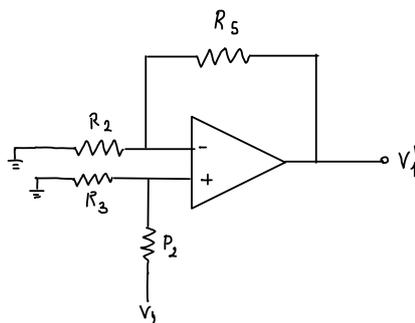
$$\left. \begin{aligned} V_+ &= V_- = \frac{R_3}{R_3 + P_2} V_2 \\ V_- &= V_1' \frac{R_2}{R_5 + R_2} \end{aligned} \right\}$$
