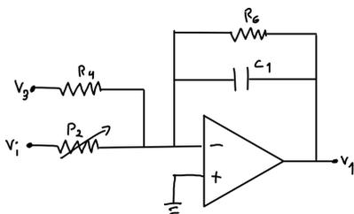
$$\frac{V_3}{R_4} + \frac{V_i}{P_2} = -\frac{V_1}{R_6 // C_1} \Leftrightarrow \frac{V_1}{\delta C_2 R_{11} R_4} + \frac{V_i}{P_2} = -\frac{V_1}{R_6} (\delta C_1 R_6 + 1)$$
