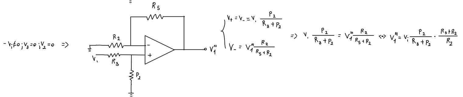
$$\Rightarrow V_1 = V_1' + V_1'' + V_1''' = \frac{R_3(R_5 + P_2)}{R_2(R_3 + P_2)} V_2 - \frac{R_5}{R_2} V_3 + V_1 \cdot \frac{P_2}{R_3 + P_2} \cdot \frac{R_5 + P_2}{R_2} = \frac{R_5 + R_2}{R_3 + P_2} \left( \frac{R_3}{R_2} V_2 + \frac{P_2}{R_2} V_1 \right) - \frac{R_5}{R_2} V_3$$
