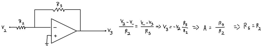
$$\frac{V_2 - V_i}{R_2} = \frac{V_i - V_3}{R_5} \Rightarrow V_3 = -V_2 \frac{R_5}{R_2} \Rightarrow A = \frac{R_5}{R_2} \Rightarrow R_5 = R_2$$
