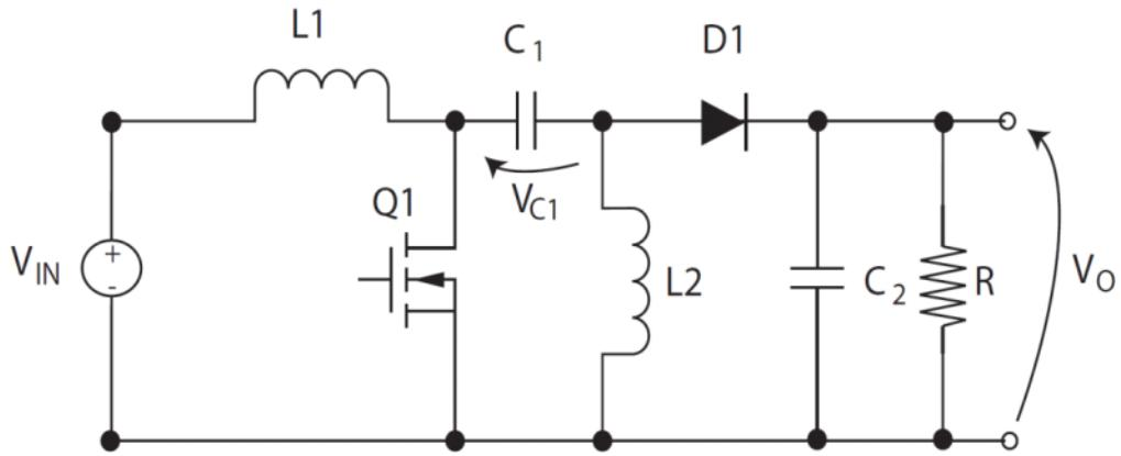
1) The DC-DC converter shown in Figure 1 operates in CCM.
