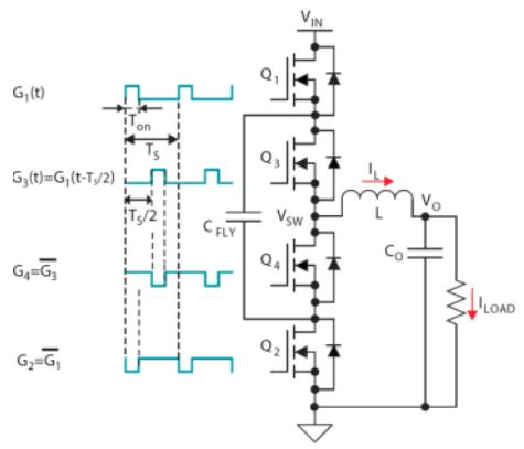
$$c) (V_{SW} - V_o)D + (V_{SW} - V_o)(\frac{1}{2} - D) = 0$$
